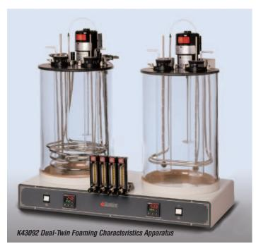
**D892 and D6082 Dual Twin Foaming Characteristics Test Apparatus**—For four tests in accordance with control ASTM D6082 and ASTM D892 specifications. Heated liquid bath features digital temperature control and an operating range to 150°C with four flowmeters to maintain the required flow rate of 94 and 200mL/min to the air diffusers. Requires the use of an external chiller to perform the Sequence I and III tests at 24°C.
