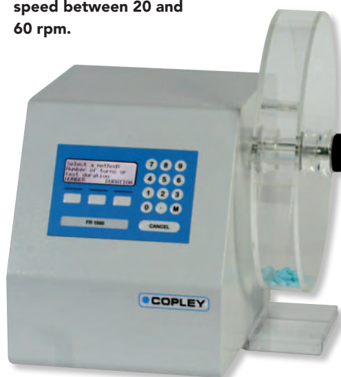
◀ Friability Tester FR 1000 (for Uncoated Tablets)
